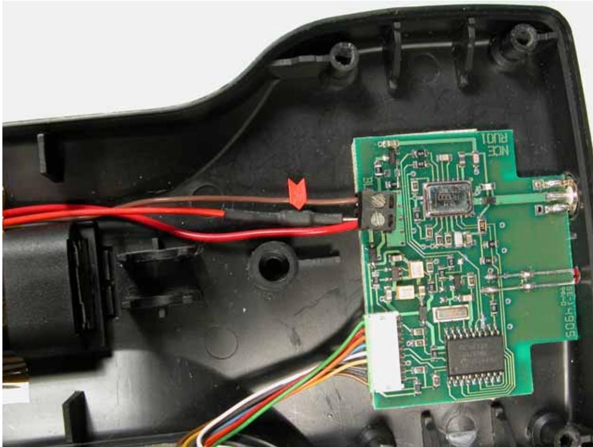
This photo shows a close up of the diode that is inline with the red wire coming from the regulator. While you can't actually see the diode because it is under the black heat shrink tubing, the banded end (cathode) of the diode should be connected to the screw terminal.
