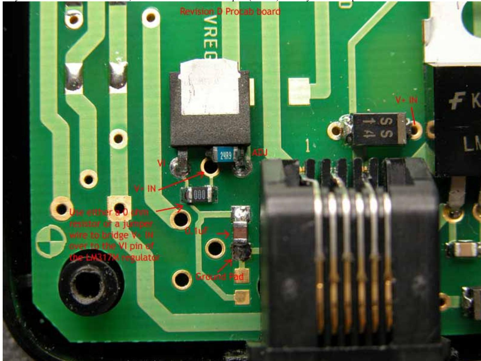
Step 4: Solder the diode across trace cut #2 as shown. Note that the banded end (cathode) should be facing the top of the Procab board as shown. Also scrape off the green soldermask just above the diode and solder a wire (red preferably) to this trace. This wire should be long enough to reach over to the battery connector on the radio board. See photo below:
