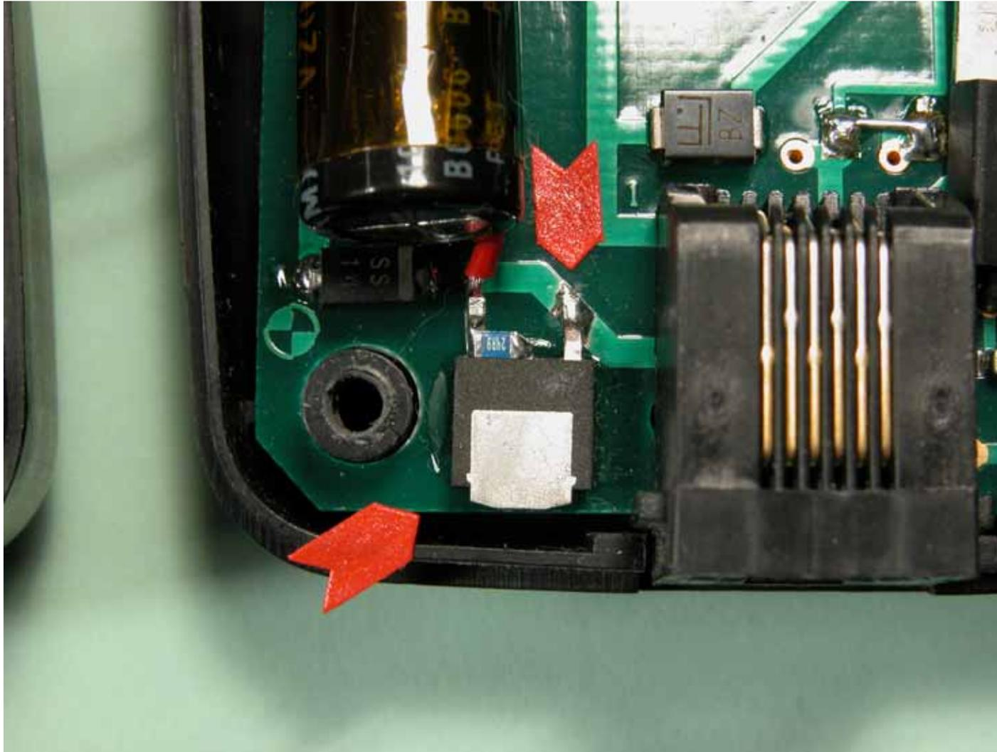
This photo shows how I connected the regulator to the angled +12 volt trace that is right next to the cab bus jack. Since only one pin is soldered to the trace I used a little bit of 5 minute epoxy and glued the regulator to the board to give it some extra support.
