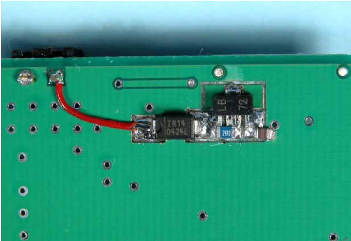
And here is a picture of the top side of the board showing where the feed through wire solders on the end of the resistor labeled 273. (at the point of the red arrow).
