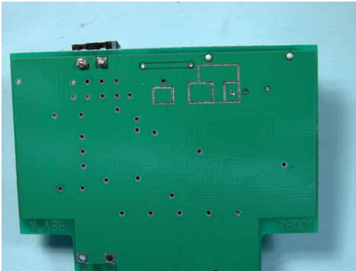
After cutting out the pads I scraped the green soldermask off the pads and drilled a hole in the center of pad on the right. This pad is the +12 volt input to the regulator and the hole is for a feed through wire that will connect to +12 volts on the topside of the PC board.
