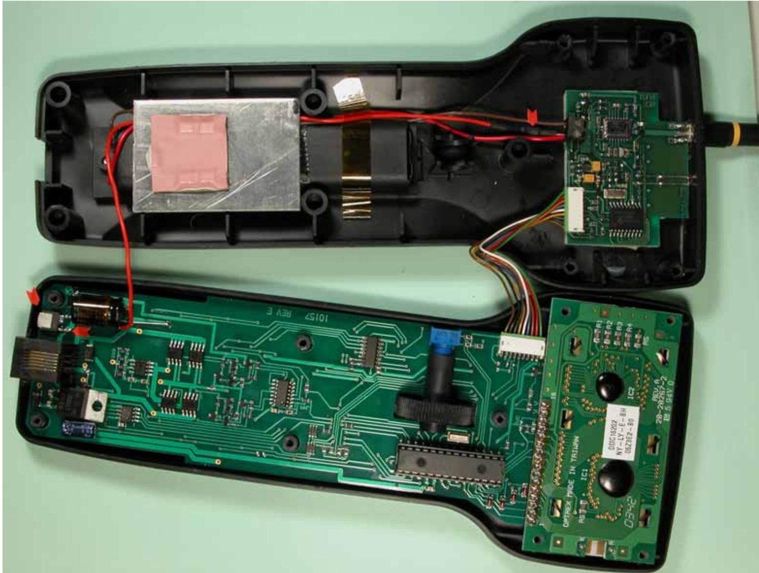
This photo shows the entire installation with the red wire connecting to positive radio board battery terminal. Since there really wasn't a good place to put the diode that needs connect to the output of the regulator I just used a leaded 1N4001 diode and wired it in line with the red wire. This is what is under the black heat shrink tubing right where the red wire connects to the positive screw terminal.
