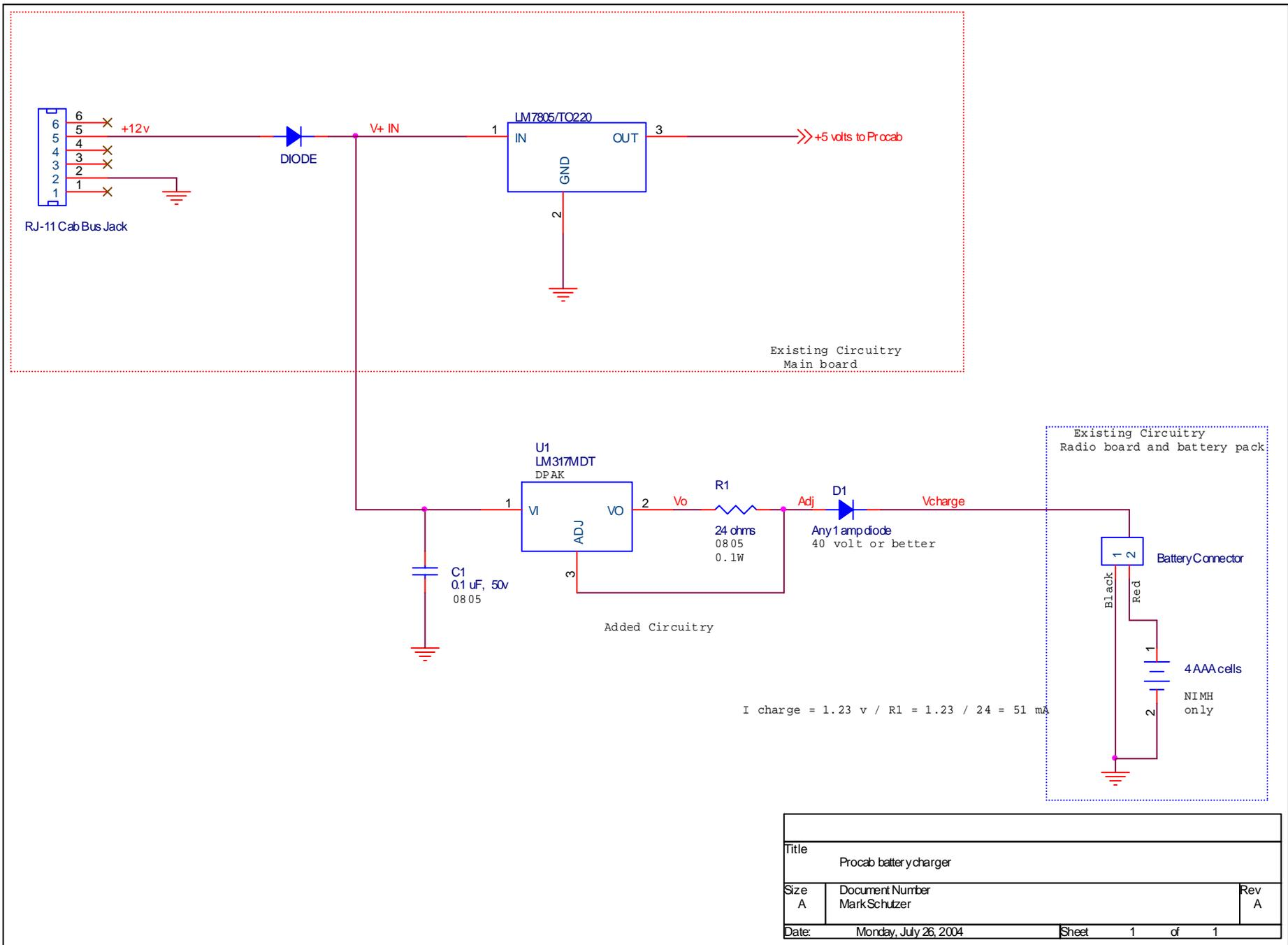
To complete the circuit description I should mention the two supporting components for the regulator. A diode has been placed in series with the charger output to prevent the battery current from flowing back into the regulator when the Procab is disconnected from the cab bus. A 0.1 uF capacitor has been placed from the regulator input to ground to filter noise and to provide stability for the regulator input. (This 0.1uF capacitor can be considered optional)
