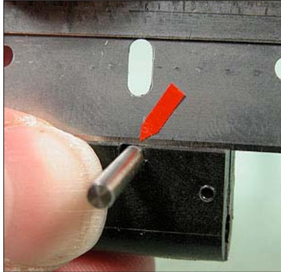
Note the gap between the axle and the bottom surface in the close up photo.
