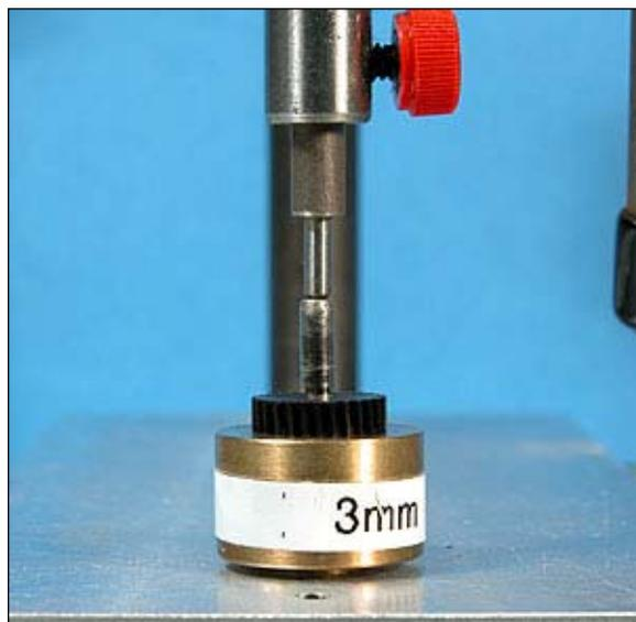
A caliper is helpful in making these measurements. If you use any Loctite be sure to clean off all the excess so that it doesn't get in the bearings.
