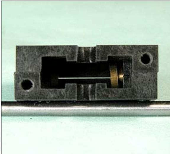
Here is a photo of a 0.4 mod gearbox showing a loose bearing that will not even stay in place.
