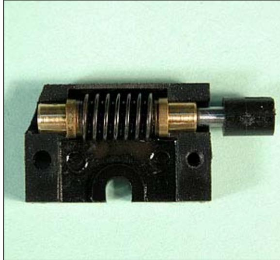
Before installing the gearbox on the driver axle I recommend that you completely reassembly all the drivers, rods, and valve gear mechanisms. Make sure that this all runs freely with out any binds before securing the gearbox assembly to the geared driver. I can't emphasize this step enough, no matter how good your gearbox is it can't make up for a mechanism that is full of binds.
