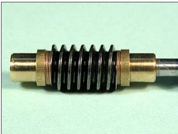
Here's a picture of the worm assembly with the thrust washers in place.
