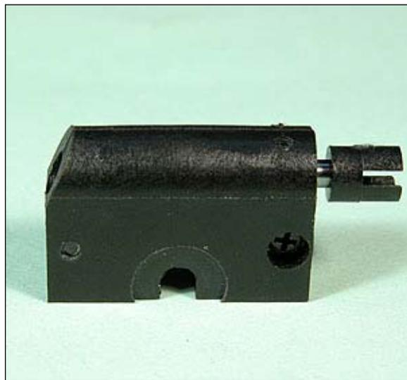
When you are happy with the performance of the driver mechanisms it's time to secure the gearbox to the geared driver. Once again lubricate the axle gear with Labelle #102 and the axle with Labelle #108. As you set the gearbox in place you should feel it snap in place. Turn the locomotive's mechanism over and install the bottom cover plate on the gearbox using the screws provided. Tighten these screws until the bottom cover is snug against the gearbox bottom surface.
